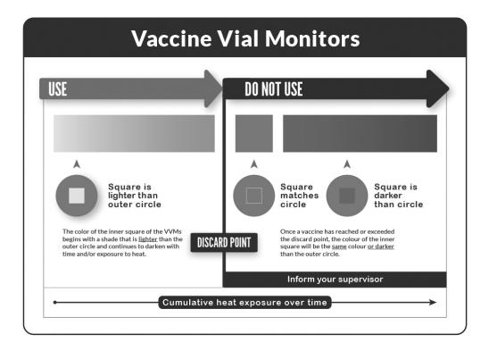
VVM is a label containing a heat-sensitive material which is placed on a vaccine vial to register cumulative heat exposure over time. The colour dot appears on the VVM label in square element is a time-temperature sensitive dot that provides an indication of the cumulative heat to which the vial has been exposed. It warns the end user when exposure to heat is likely to have degraded the vaccine beyond an acceptable level.
